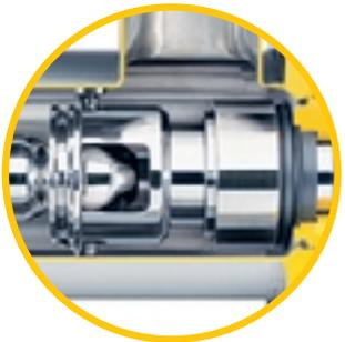
**Suction Casing** made of stainless steel, internally polished externally satin finished. "Dead zone free" design with suction connection above the mechanical seal enables CIP solutions to flow through the entire casing. Choice of off-set CIP-connection for residue-free cleaning and complete draining. Options with jackets for heating. Standard connections according to DIN 11851, 11864 or Tri Clamp®.
